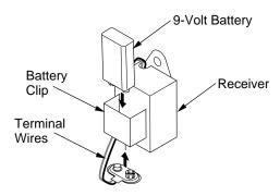
Figure 16 - Installing Battery in Receiver
